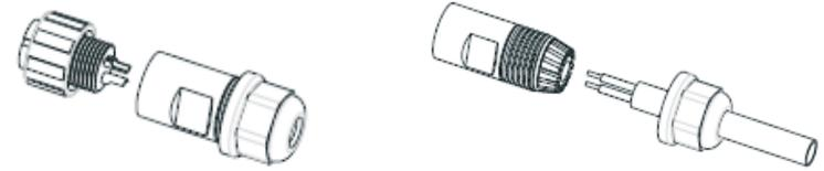
2. Make the RS485 cable go through the connector.
